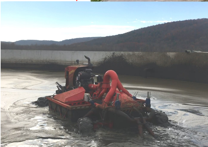
Agitation boat used to get manure solids and bedding in suspension for field application — specifically suited for sand or very large storages.
