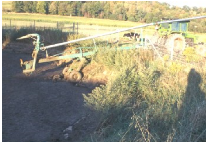
Agitation boat used to get manure solids and bedding in suspension for field application — specifically suited for sand or very large storages.
