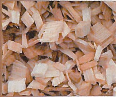
Large woodchips are important for woodchip pad longevity and drainage. (Photo: David DeVallance, West Virginia University, Wood Science and Technology)
