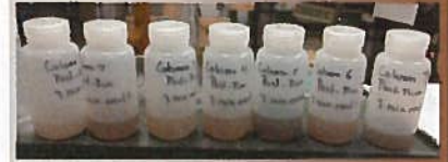
Water samples taken from woodchip pads using a variety of different types of woodchips. (Photo: David DeVallance, West Virginia University, Wood Science and Technology)
